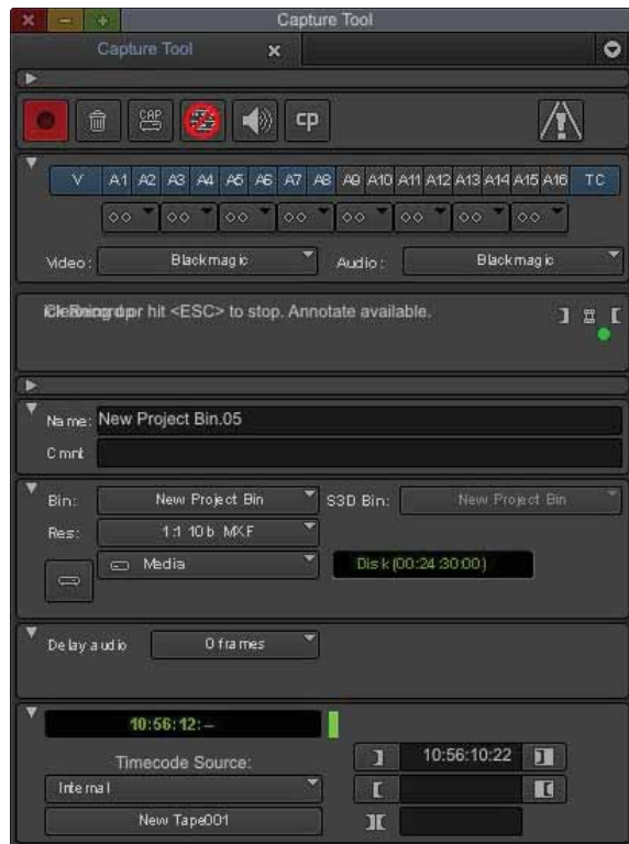
Step 2. Set up the Capture Tool to capture video by clicking the Toggle Source button.
