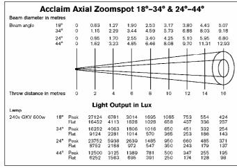
Tests conducted using a standard GKV, 600W, 240V, lamp.
