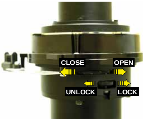
Figure 3-24 Aperture Manual Adjustment
